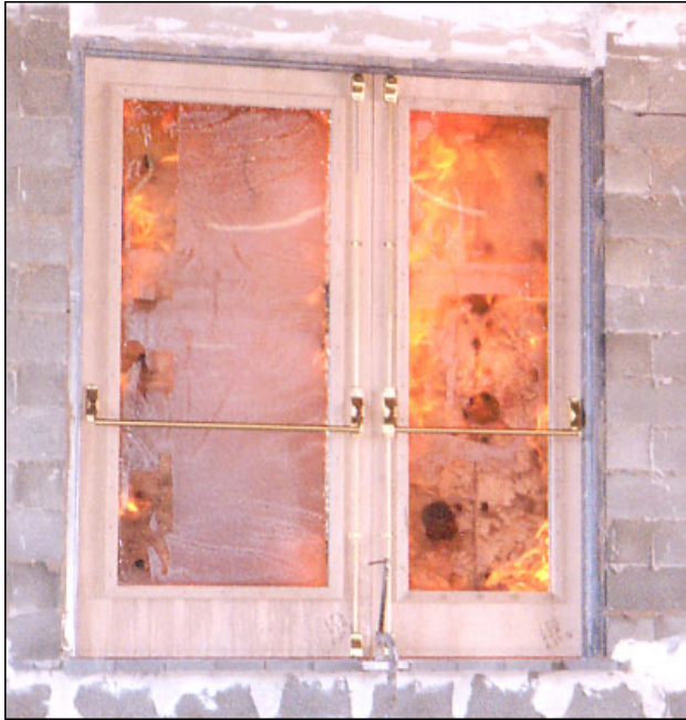
Glass exposed to fire
